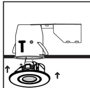
STEP 3 : Connect the wires using quick connect system.
