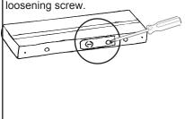
B.Remove appropriate 3/8" diameter knockout for supply wiring entry
