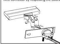
G. Replace the plate back on the light and tight it with screw and mount fixture (see mounting section)
