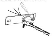
F. Attached each wall cable to the light Wire connector by respecting the colors
