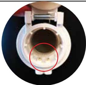
If the pins, once pushed, do not come up; the spring is probably broken and could cause the vacuum not to start or stop. In which case the spring must be fixed.
